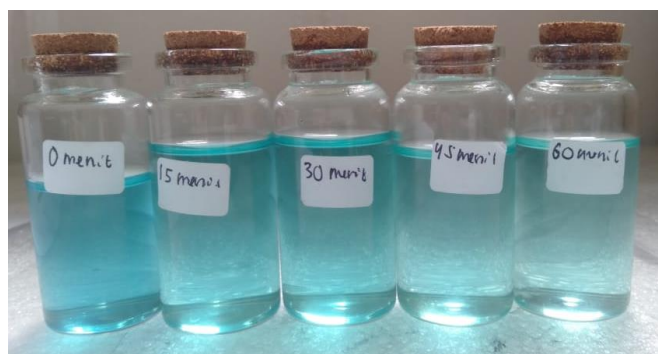
Figure 5. Visual comparison of batik wastewater samples treated with ozone over different exposure times.
